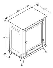
Figure 1 - Heater Dimensions
